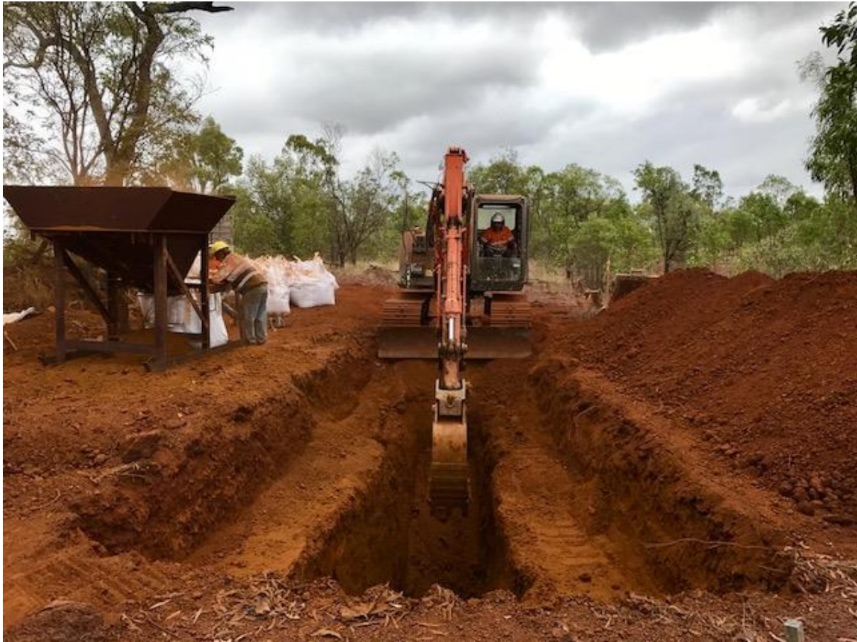
Figure 1: Trial mining operations have commenced at the Sconi Cobalt-Nickel-Scandium Project in northern Queensland to collect a 20 tonne bulk sample to run through the Company's demonstration-size plant currently being constructed in Perth. Note that as the ore body outcrops, the first buckets of dirt extracted at Sconi are actually cobalt and nickel-rich ore. Thus, there is almost zero stripping required at Sconi for this initial operation.
