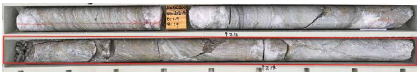
Figure 5 - Photo of AKDD200 drill core including a highlighted section of the mineralised interval: 1.0 m @ 2.2% Pb, 8.3% Zn (10.5% Pb+Zn), 250 g/t Ag and 0.2 g/t Au from 213.4 m.
