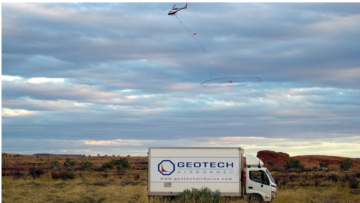
Figure 2: Airborne electromagnetic (AEM) survey in progress (Photo taken by UTS crew)
