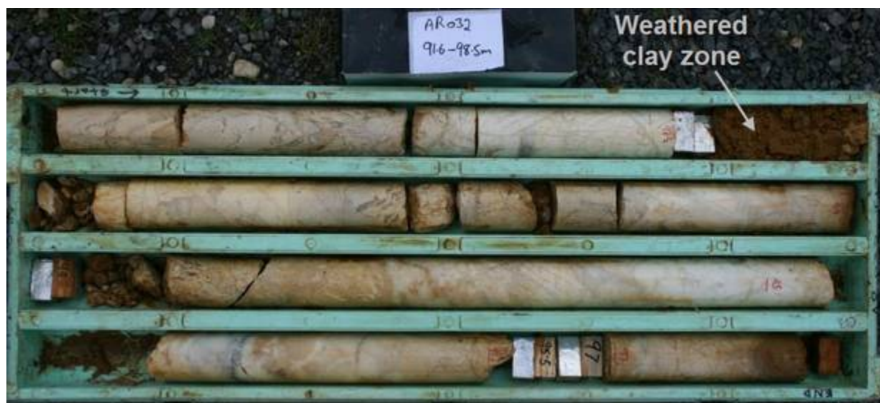
Figure 26: Weathered zone in AR032 – 92.5m
