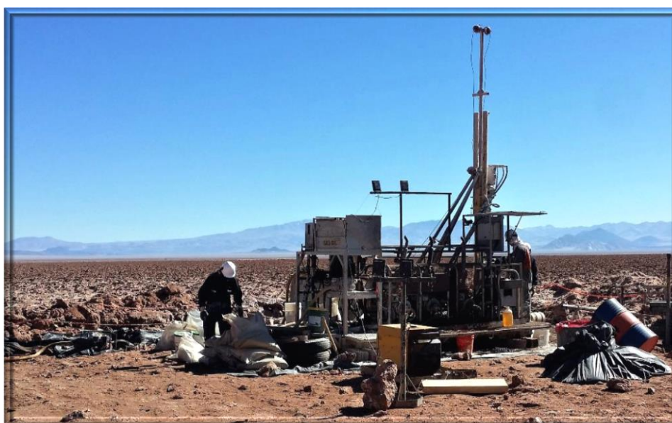
Images of the diamond drill rig at the first and second drill holes of the Kachi project
