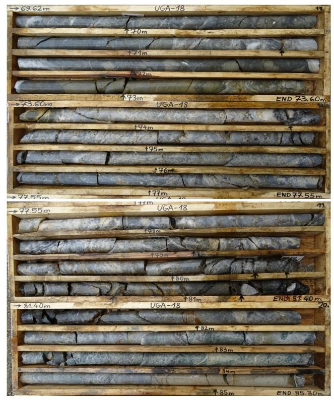
Figure 4: UGA-18 drill core; part of the interval from 45m to 82.7m (down-hole) showing quartz filled vein/stockwork/breccia structures, variably rich in fine to very fine grained sulphides (mainly pyrite/marcasite) and hosted within strongly argillic altered andesite host rock. Traces of visible gold identified at 81.35m
