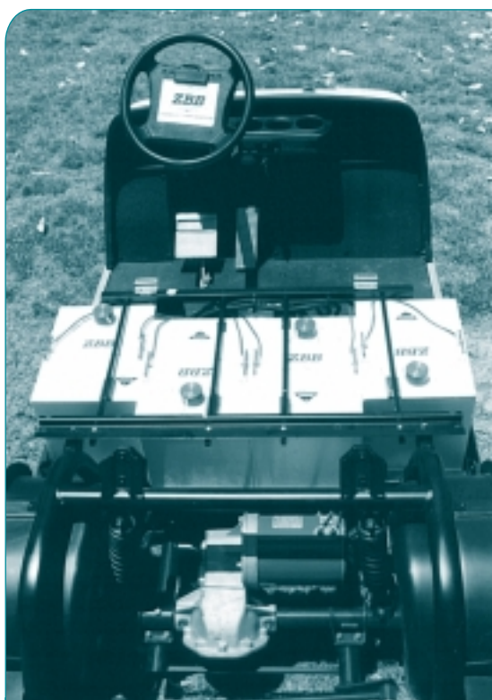
Four (4) ZBB non-flow batteries in test bed golf car
