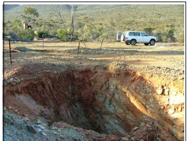
Mt Desmond Drill Site looking north, showing copper oxide mineralisation in the collapsed working. Old ventilation infrastructure is evident at the rear of the shot.
