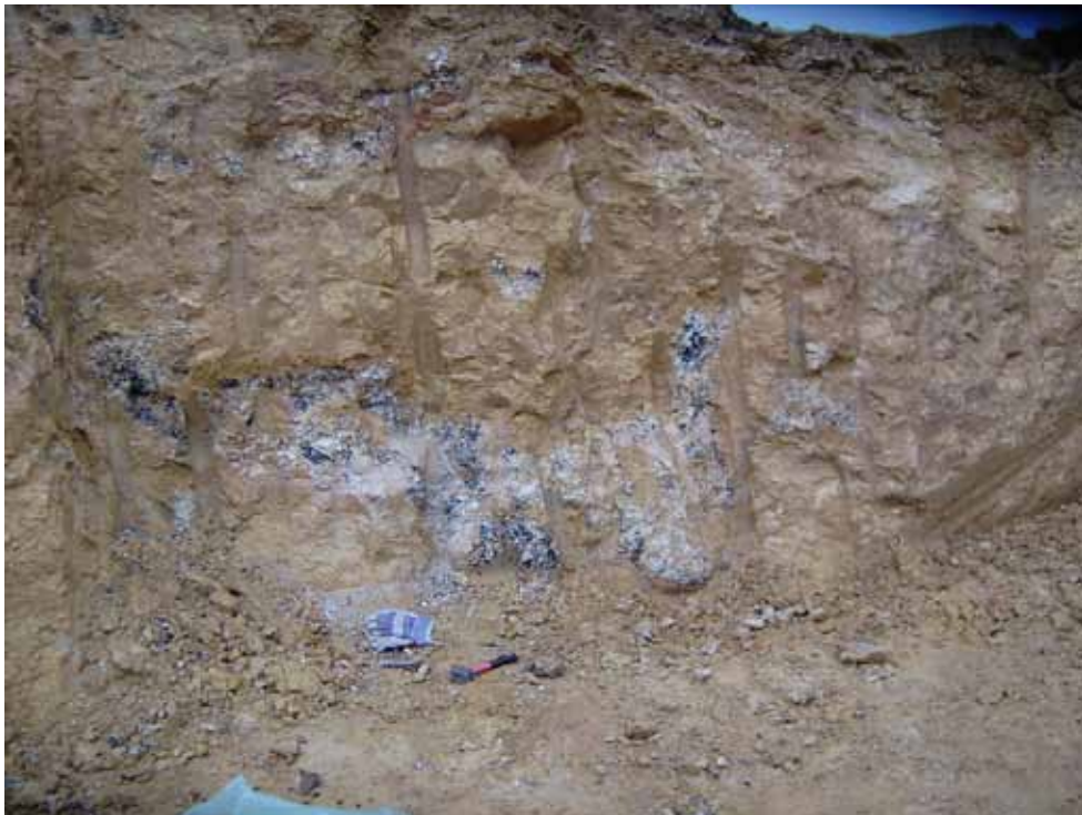
Figure 13 Phosphate associated with manganese oxides in the current Tarcowie Phosphate Pty Ltd operation near Tarcowie.
