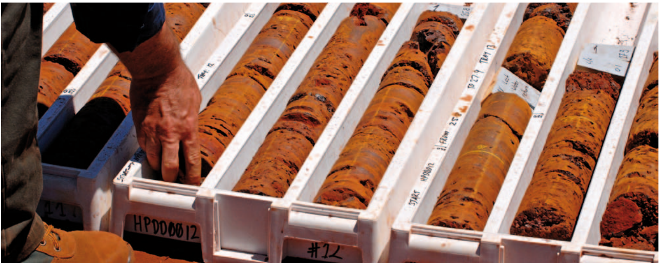
Drill core trays containing the PQ (83mm) diameter metallurgical core of BID mineralisation.
