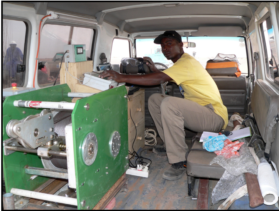
Figure 3: Photo of Log Operator recording down-hole gamma readings during the current drilling program
