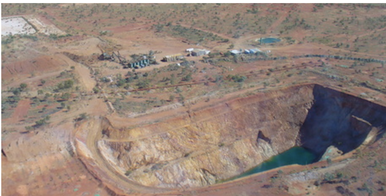
Nicolsons Mine, the focus of works at Halls Creek, with open pit in the foreground, processing plant and surface facilities centre, and existing tailings facility at top of picture.
