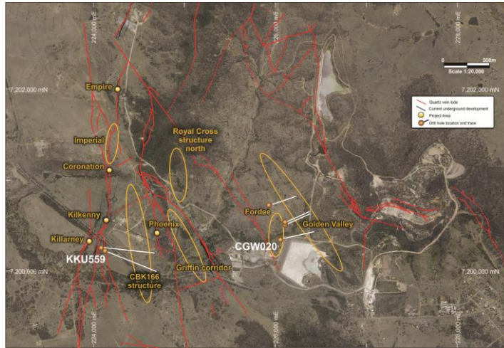
Cracow regional location plan showing referenced prospects, lode structures and drill hole locations
