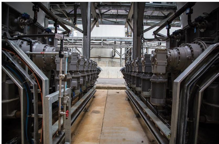
*Reclaim discharge screw conveyors at base of DiCOM vessels.*
