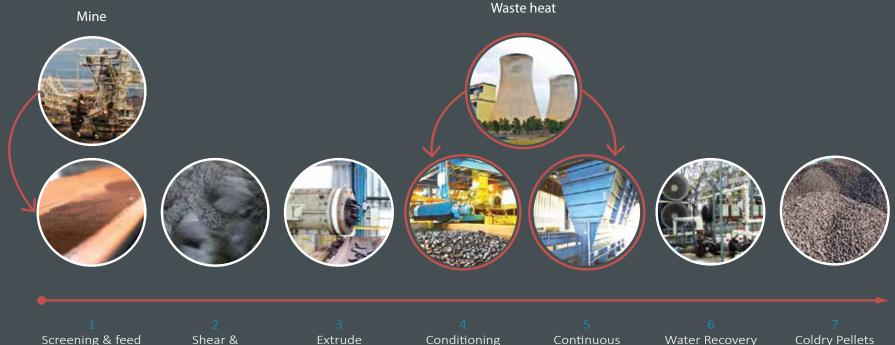
Primary processing begins when brown coal is mined and delivered to the Coldry plant where it is milled and screened to achieve a consistent
