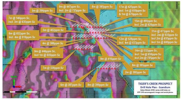
**Figure 2:** 2018 Drill Hole Plan – Best Scandium intersections<sup>2</sup>
