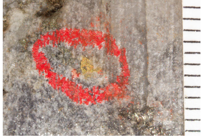
Figure 11. Free gold and sulphide at 264.80m in TGGRCDD110 (scale: mms).
