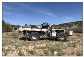
Seismic buggy drill machine
