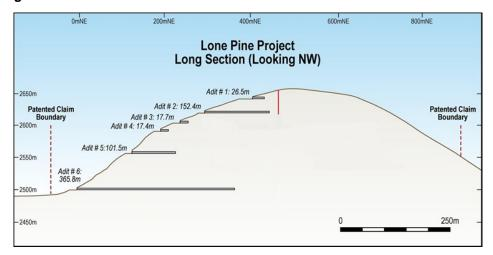
Figure 5 - Lone Pine Vein Zone - Long Section Looking NW (plane of vein)
