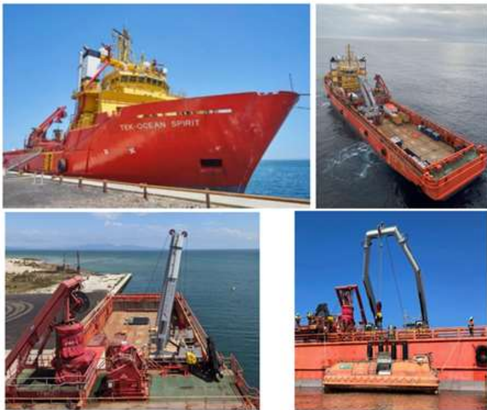
The TEK-Ocean Spirit has been upgraded to allow it to transport and operate Remotely Operated Vehicles (ROV) along with a third-party owned 45Te Hyperbaric Rescue Vessel (HRV) A-Frame lifting mechanism, both of which allow the TEK-Ocean Spirit to undertake broader subsea support operations. Further modifications are underway in dry dock in Singapore.
