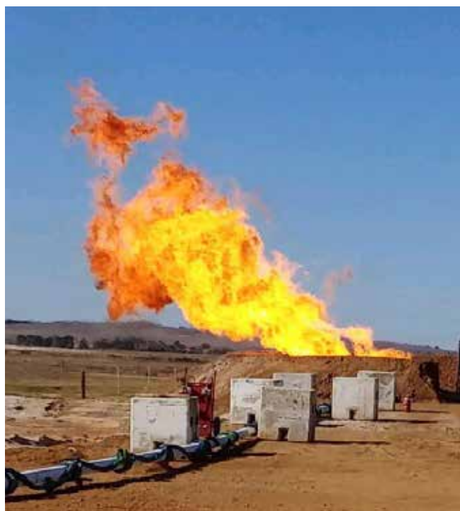
Flow Testing D Sands at Walyering-5
