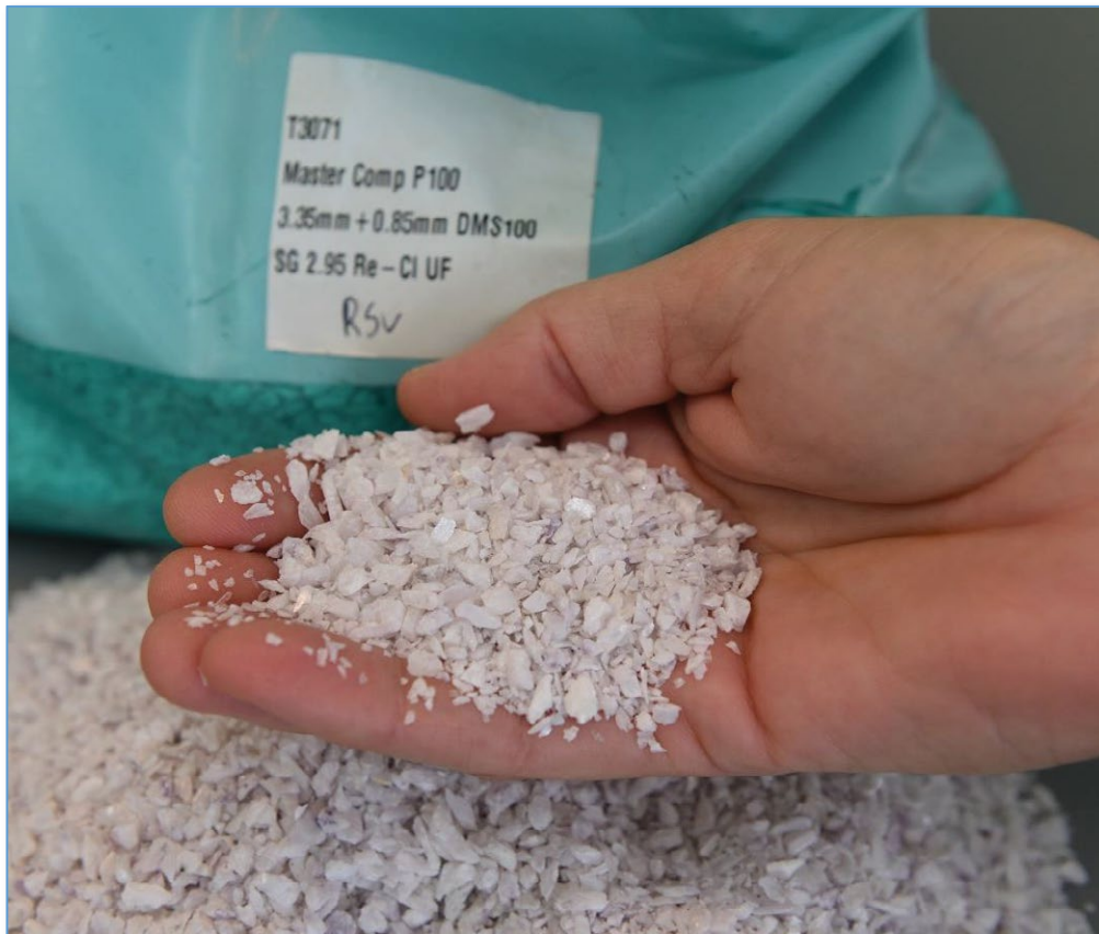
FIGURE 4: HIGH PURITY SPODUMENE DMS CONCENTRATE (SC 6.5) PRODUCED FROM 3.35MM+0.85MM DMS 2.95 FEED
