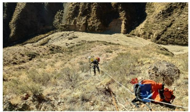
Figure 1: Field workers placing electrodes
