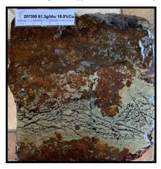
**Photo 1c** High grade chalcopyrite-garnet-magnetite polished rock sample from Leah's Lode outcrop, 2m from trench - 61.3g/t Au, 18% Cu, 135g/t Ag<sup>2</sup>.
