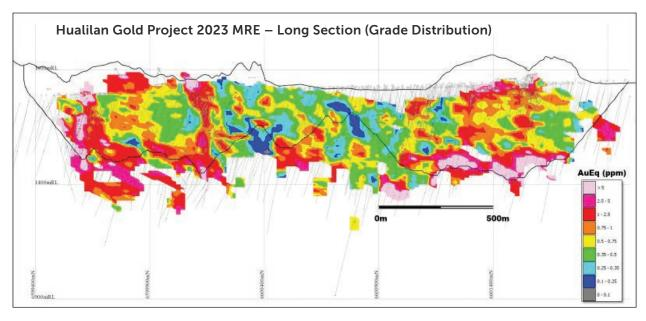
Figure 3 – Long Section of the upgraded MRE showing grade distribution in
