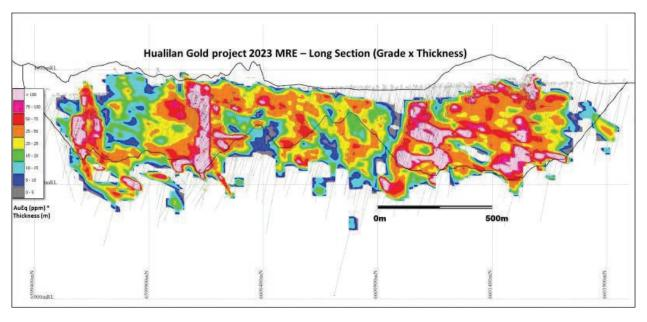
Figure 2 – Long Section (MRE block model)
