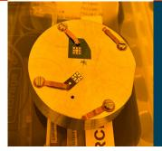
Archer's biochip innovation aims to integrate graphene field effect transistors ("gFETs") into advanced fluidic systems to create miniaturised lab-on-a-chip device platforms for medical diagnostics.
