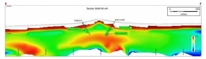
*Figure 11.* East-West section through the Sugarloaf Graphite Prospect – Eyre Peninsula, South Australia
