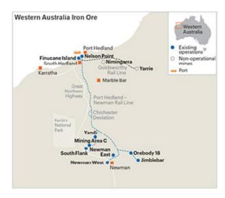
Western Australia Iron Ore (WAIO) is an integrated system of four processing hubs and five open-cut operational mines in the Pilbara region of northern Western Australia, connected by more than 1,000 kilometres of rail infrastructure and port facilities.
