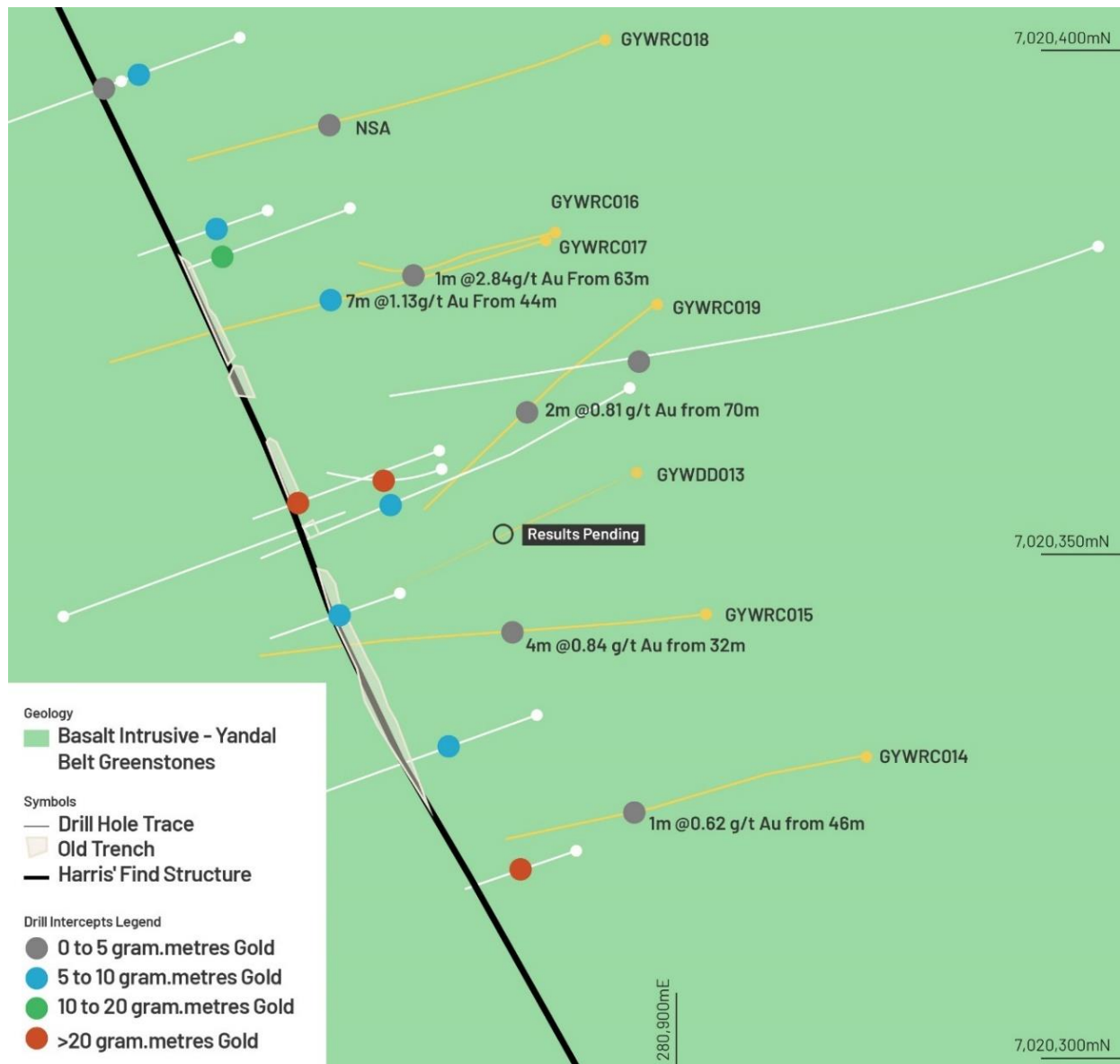
Figure 20: Plan section of reported drill-hole results positions.
