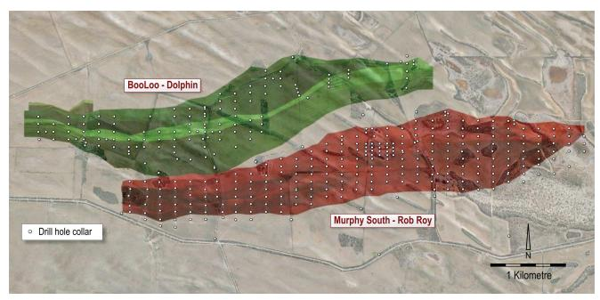
The CEIP orebodies have been extensively and systematically drilled along north-south traverses defined by a notional 200x100m diamond drill spacing.
