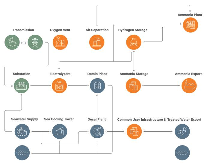
Upstream power and Cape Hardy green hydrogen precinct anhydrous ammonia block flow schematic (source AMP Energy).
