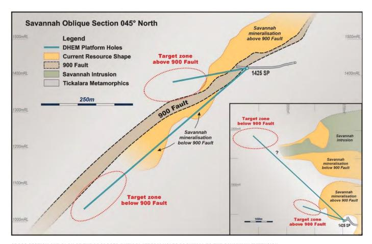
CROSS SECTION AND PLAN OF THE PROPOSED DHEM PLATFORM HOLES PROXIMAL TO THE SAVANNAH EXTENSION
