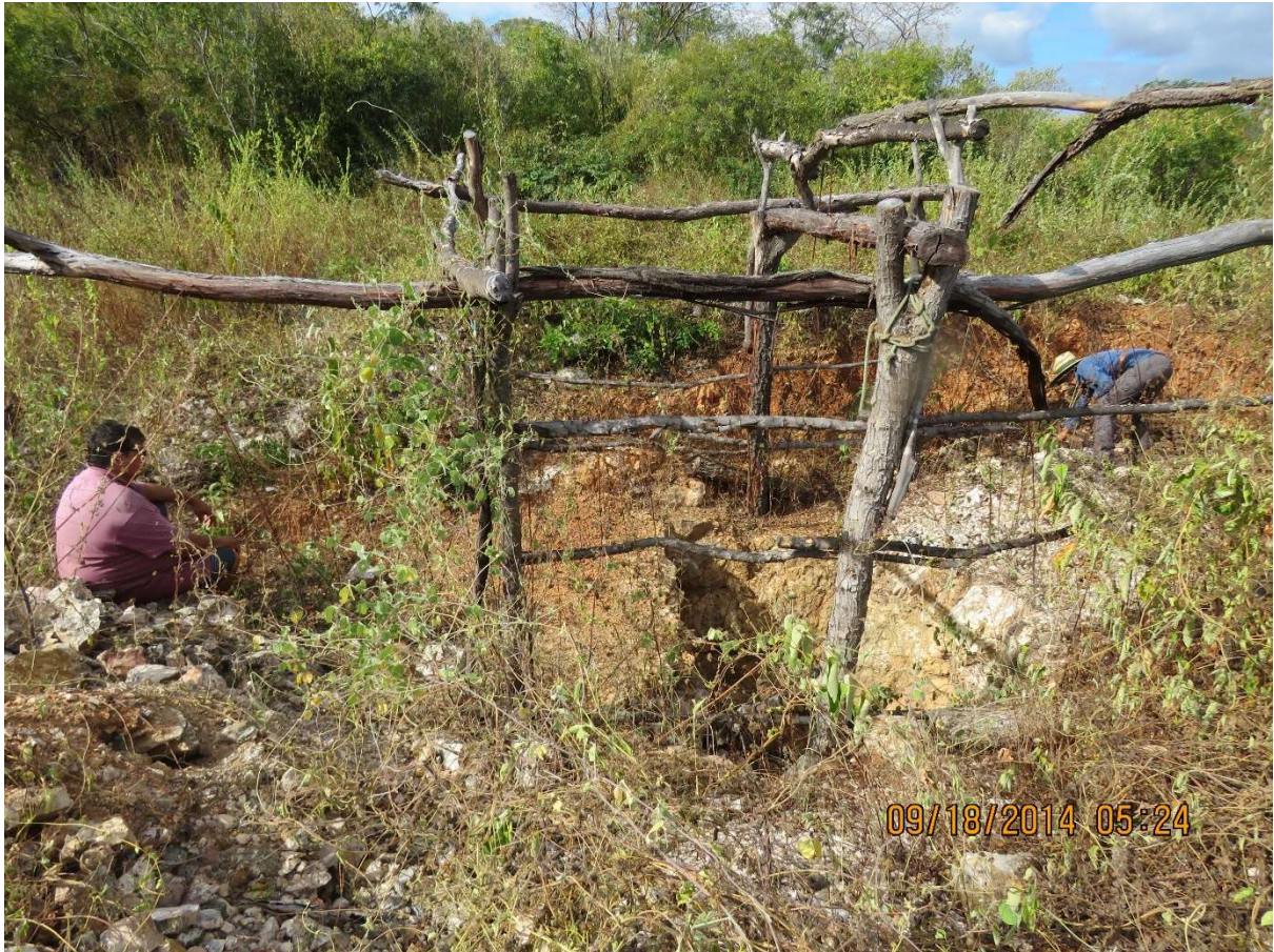
Figure 7. Small shaft at Ico. Pegmatite had abundant perthitic feldspar, a quartz core and areas with small and large muscovite books. Beryl was present and was the reason the shaft was excavated initially. Farmer/garimpeiro sitting on the edge of the waste dump.
