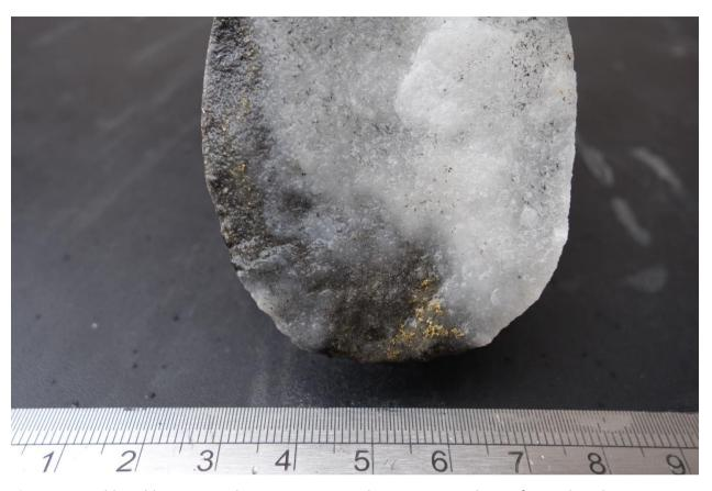
**Figure 13:** Visible gold is preserved as up to ~1cm sized aggregates made up of many less than 0.5mm grains within a ~1cm thick, translucent-white, drusy quartz veinlet at ~127.55m in UGA-52.
