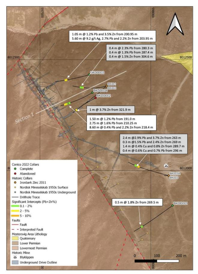
Figure 6 Plan map of 2022 and historic drilling at the Blyklippen historic mine, showing significant intercepts (non-verified historical intercepts in grey boxes).
