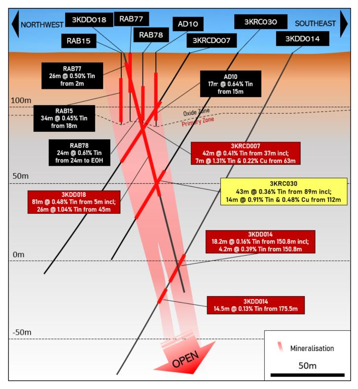
Figure 8: 3KEL Target – Cross section of 3KRCD007, 3KDD014, 3KDD018 and recent hole 3KRC030, recent results are in yellow.
