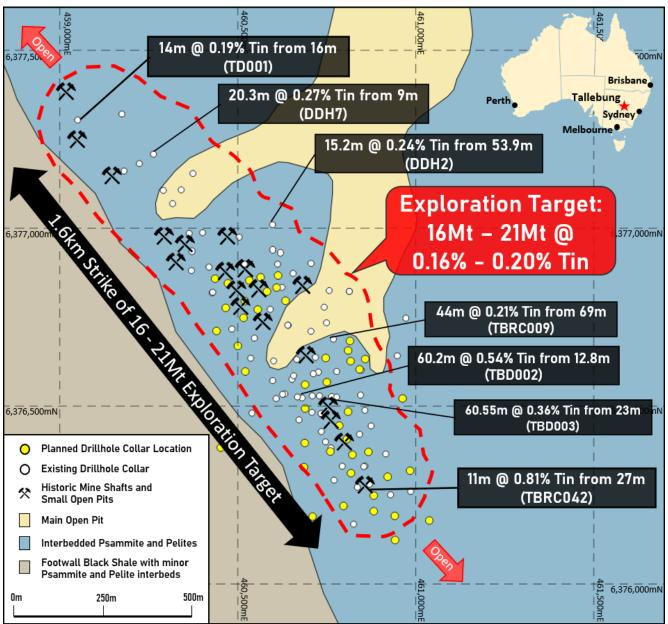
*Figure 2:* Tallebung Tin Project – Plan view showing the past drilling with highlighted intercepts, the extent of the current Exploration Target and maiden MRE, along with the locations of the planned drillholes in the resource expansion and infill drilling program now commenced overlaid on the geology.
