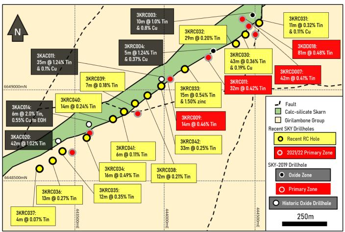
*Figure 7:* 3KEL Target – Plan view of the southwestern end of the 3KEL Target showing the past drilling with the recent RC drillholes. Recent results are in yellow, past results in red and black for oxide and primary intercepts, respectively.
