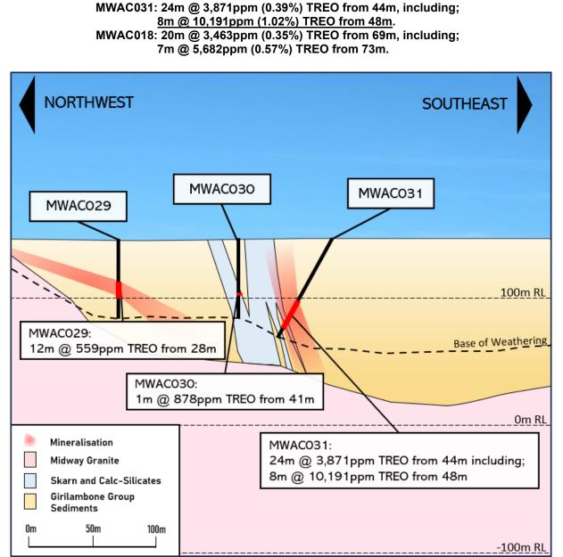
*Figure 10:* Doradilla Project – Cross-section from MWAC029 to MWAC031 showing the DMK line Skarn above the Midway Granite with the Midway Granite coming to surface and outcropping to the northwest.
