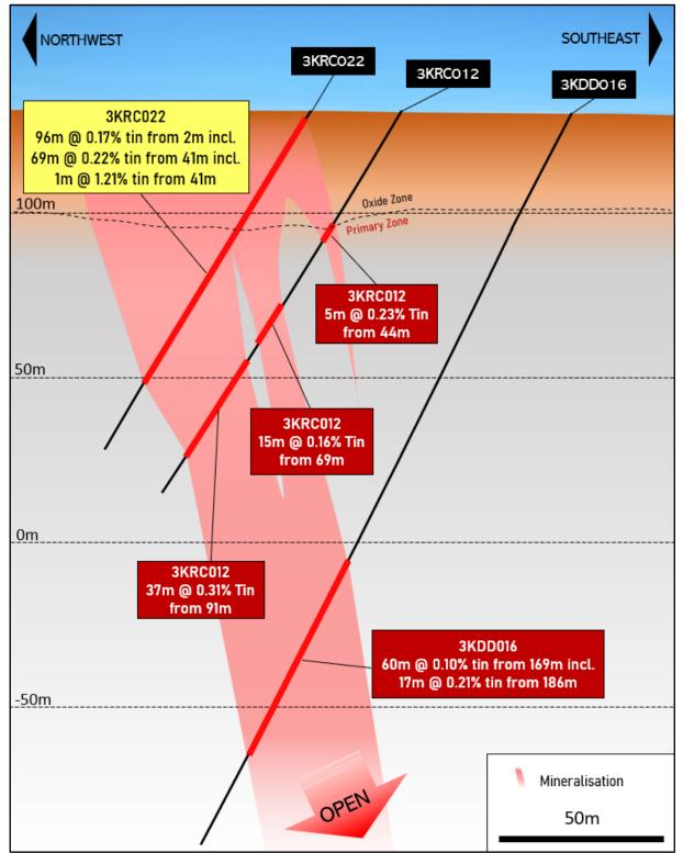
Figure 6: 3KEL Target – Cross section of 3KRC012, 3KDD016 and recent hole 3KRC022, recent results are in yellow.
