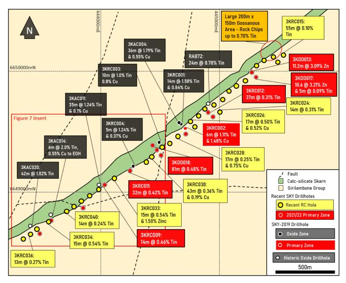
*Figure 4:* 3KEL Target – Plan view of the whole 3KEL Target showing the past drilling with the recent RC drillholes. Recent results are in yellow, past results in red and black for oxide and primary intercepts, respectively.
