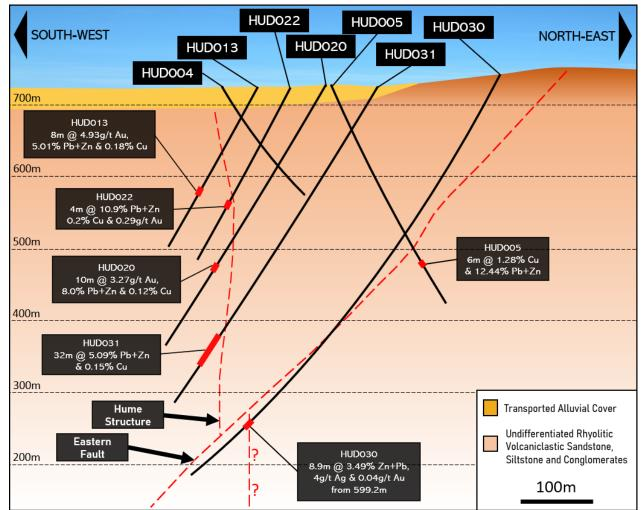
**Figure 13**: Hume Target – Cross-section of **HUD030** showing the trace in red of the extension of the hole to test the Hume Structure at depth and provide a platform for DHEM – Assays are pending for the extended hole interval shown in red.
