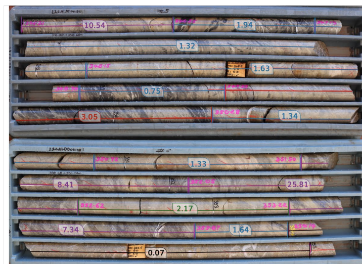
Fig 5: Calypso HQ diamond core 22 CALD011W1 with grade (g/t) intervals from 346.21m to 355.0m
