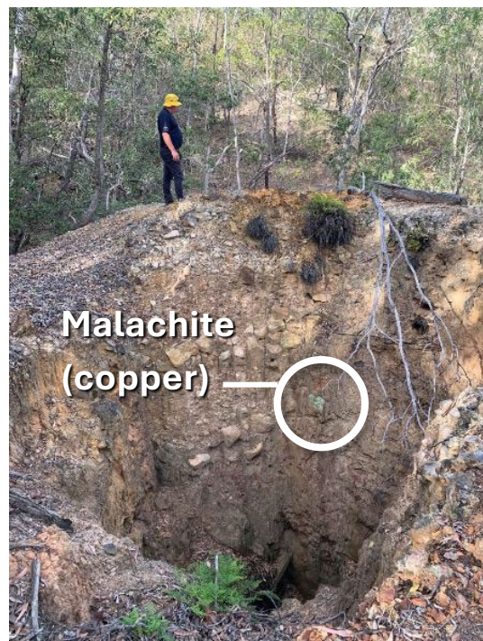
Figure 6. New shaft Identified 620m south-east of the old workings. Visible malachite in the wall of the shaft, with vertical depth of shaft estimated at 60m 18 .
