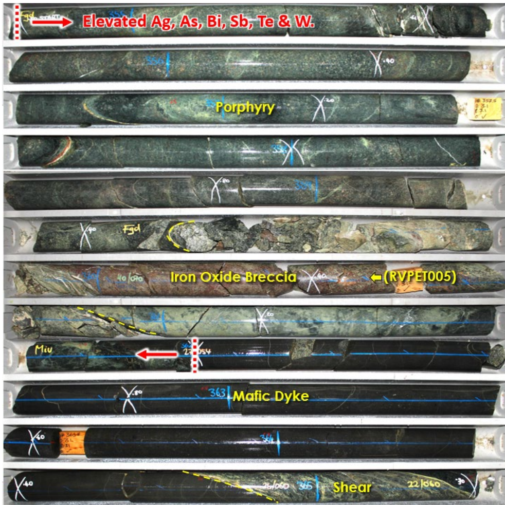
Figure 8. 7.2m zone of interest within diamond core (RVCD0006), 354.8 – 362m, containing a porphyry, iron-oxide breccia, and a mafic dyke. Multi-element assay results returned 7.2m @ 0.32g/t Ag from 354.8m 16 .
