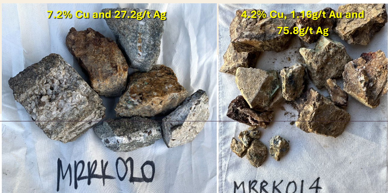
Figure 1. Rock chip sample MRRK020, bornite crystals, 1cm x 0.5cm in size, within quartz veins, at the contact between a mafic and a granite unit. MRRK014, iron rich quartz vein at surface 18
