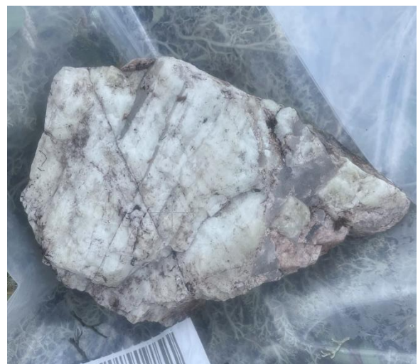
Figure 2 (top left): Photo of sample H909418 from Polaris. Photograph field of view contains 80% white to pinkish stained spodumene (SPD), 20% translucent quartz and feldspar. NB: UV light is 9cm for scale.
