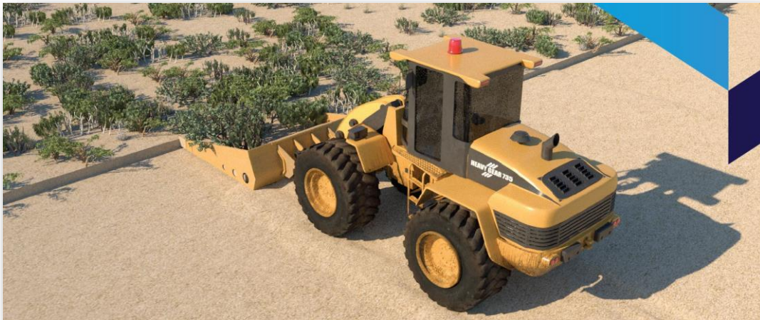
Figure 5: VDT Modified Loader Bucket
