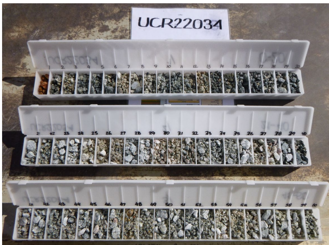
Figure 31: Phase 1 drilling programme Spodumene Pegmatite intersection RC sample.
