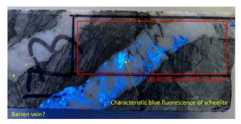
Figure 19 - Barren Vein next to a High Grade Vein.
