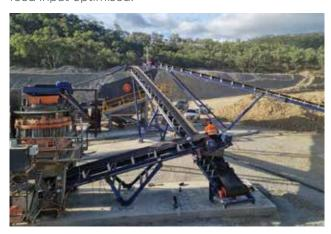
Crushing and Screening Plant with the Cone Crusher at the forefront.
