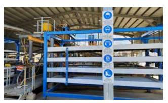
Eight additional shaker tables have been installed and commissioned to increase processing capacity.
