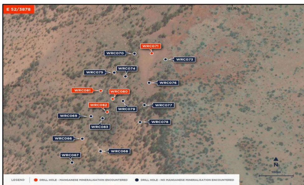
Figure 4 - Drill hole location plan showing location of Phase 2 RC drill hole with Manganese mineralisation at Mn Area 4
