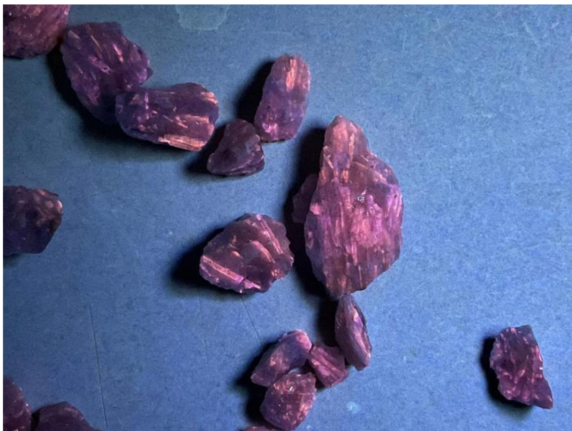
Figure 12: Spodumene crystals in HYRC006 (162-163m) under 250nm ultraviolet light (1m @ 0.47% \text{Li}_2\text{O} )
