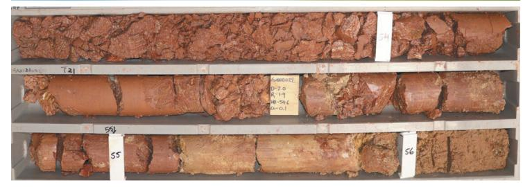
Above photo: Narraburra REE Diamond drillhole GNBDD0022 4m @ 2,354ppm TREO from 52m, inc 2m @ 4,494ppm from 52m
