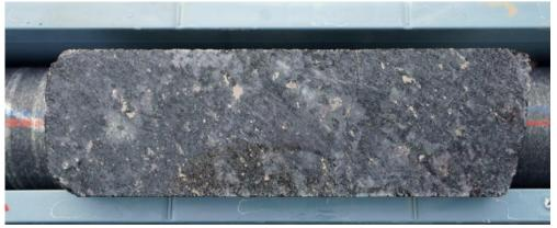
Figure Two | Disseminated sulphide bearing core from hole PS412
