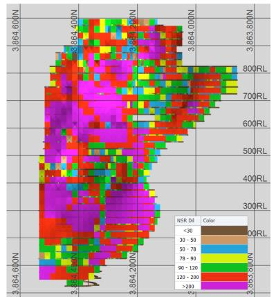
Figure 6: Long-section showing NSR value (US\$/t) of stopes – viewing from west to east.
