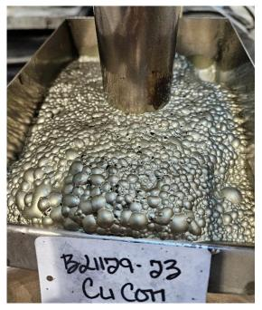
Flotation of copper during initial locked cycle test work
