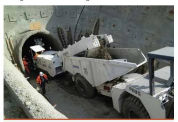
Figure 7: ITC loader paired Paus bi-directional haul trucks to be used in the trial mining
