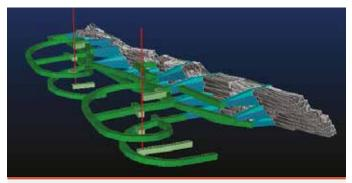
Figure 5: Conceptual layout of the +105 Mineral Resource drift-and-fill mining method
