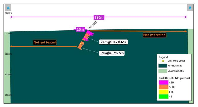
Figure 5: Cross section of OURC001 - The entire hole was mineralised other than a 4m wide felsic dyke - Only 25m of the 380m width was drill tested
