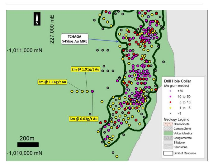
Figure 13: Tchaga West - Select new intercepts – Note the drill intercept returning 6m at 6.03g/t Au which is 200m west of the current Tchaga resource
