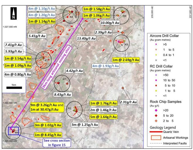
Figure 15: Komboro Prospect: Drill targets K1 to K7 – Select new (yellow) and previous (white) RC results and previous AC results (blue) and rock chips (white italics)
