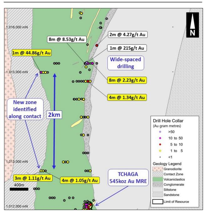
Figure 14: Tchaga North – Select new (yellow) and previous (white)drill intercepts – Note the newly discovered mineralisation at the granite/ volcaniclastic contact zone (grey striped)
