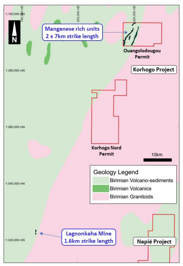
Figure 10: Size comparison of Mako's Mn-rich units compared to the footprint of the Lagnonkaha mine<sup>4</sup>
