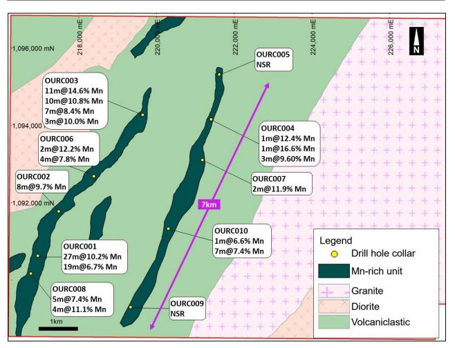
Figure 3: Ouangolodougou Permit with reconnaissance drill hole location and results. There is only one drill hole at each location and that average drill hole spacing is over 1km apart.
