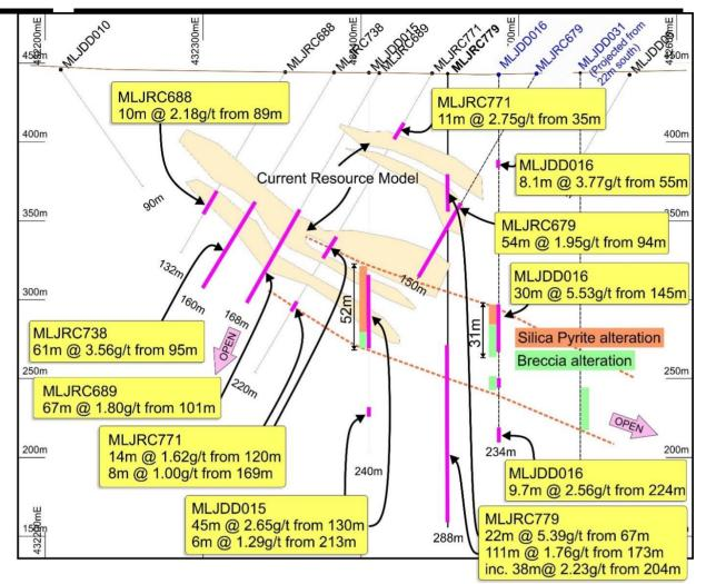
Figure 2. Composite cross section for LJN4 centre area showing thickened high-grade dipping gold zone containing breccia and silica-pyrite alteration, upper mineralised zone, older resource model outline and potential depth extensions at depth, downdip and to the east.
