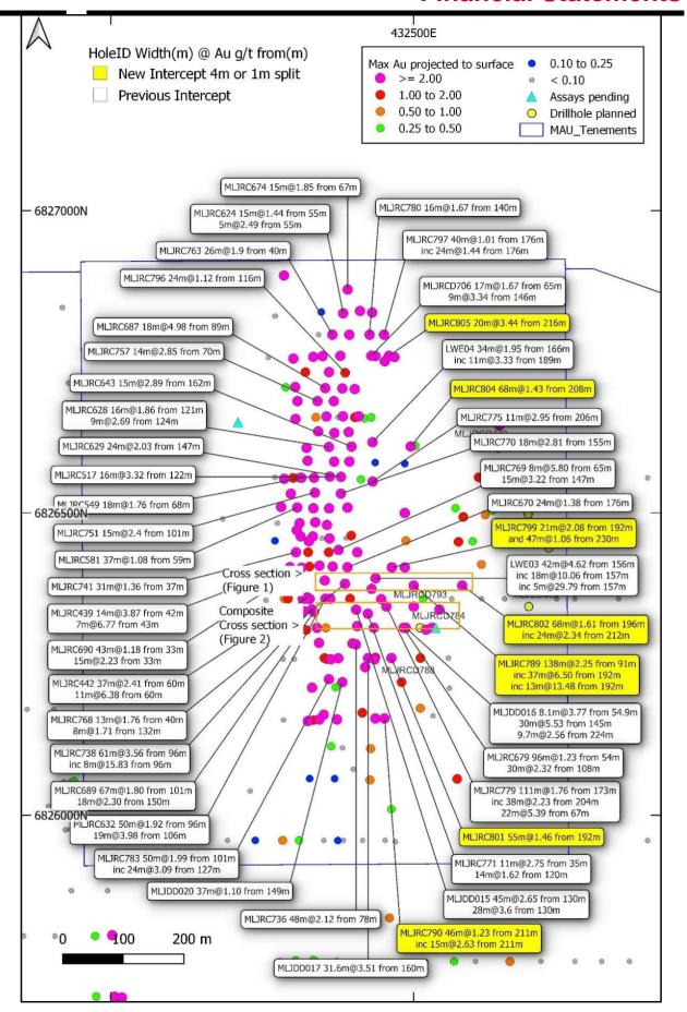
Figure 4. The Lady Julie North 4 deposit has numerous significant thick intersections from the latest drill programmes (yellow is the latest drill programme) and previous drilling (white label) with maximum gold projected to surface.
