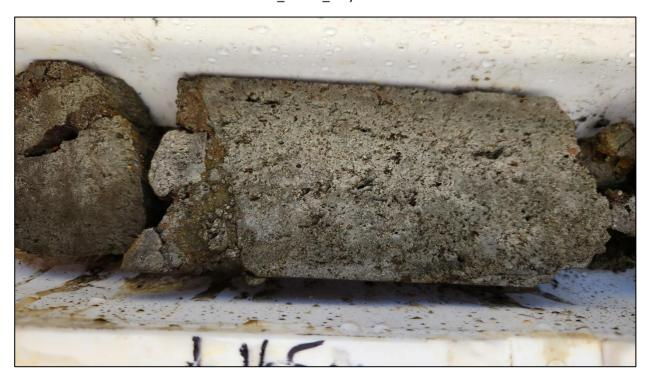
MLJDD018\_164.5m\_Massive pyrite in Breccia
