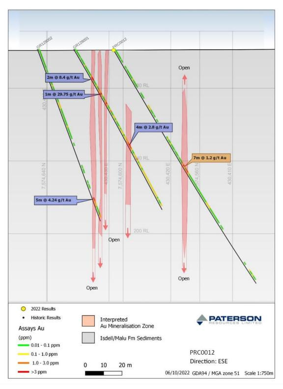
Figure 8. Cross section PRC0012 with historic drilling
