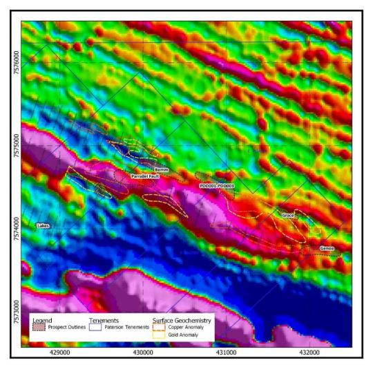
Figure 5: Coincident copper and gold anomalism overlaying aeromagnetics
