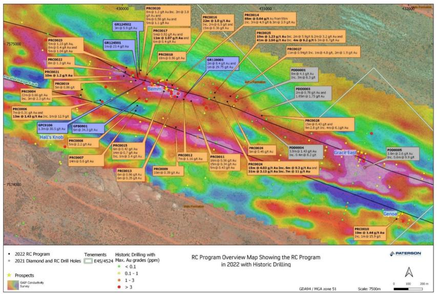
Figure 6. Overview map showing all holes drilled with their significant intercepts with historic drilling. Orange boxes show results of the recent 2022 RC drilling program,
