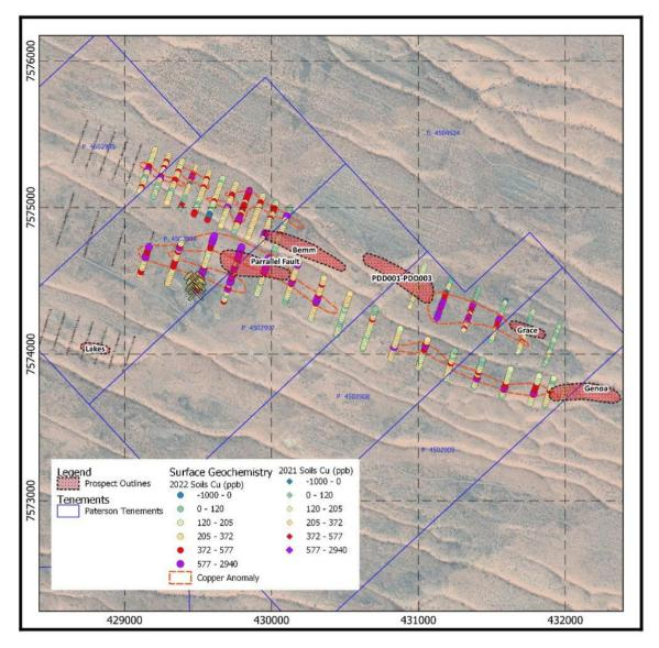
Figure 4: Copper anomalism defined by MMI soil geochemistry
