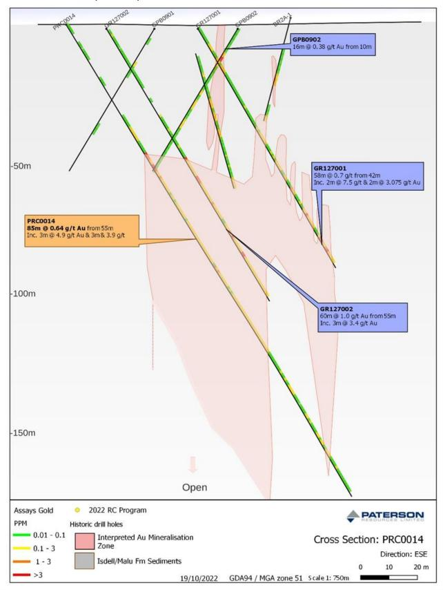
Figure 9. Cross Section with PRC0014 with historic drilling
